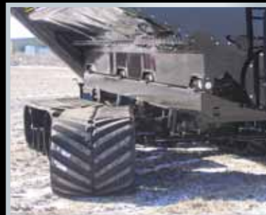
Patented Steerable Axles with Hydraulic Suspension
